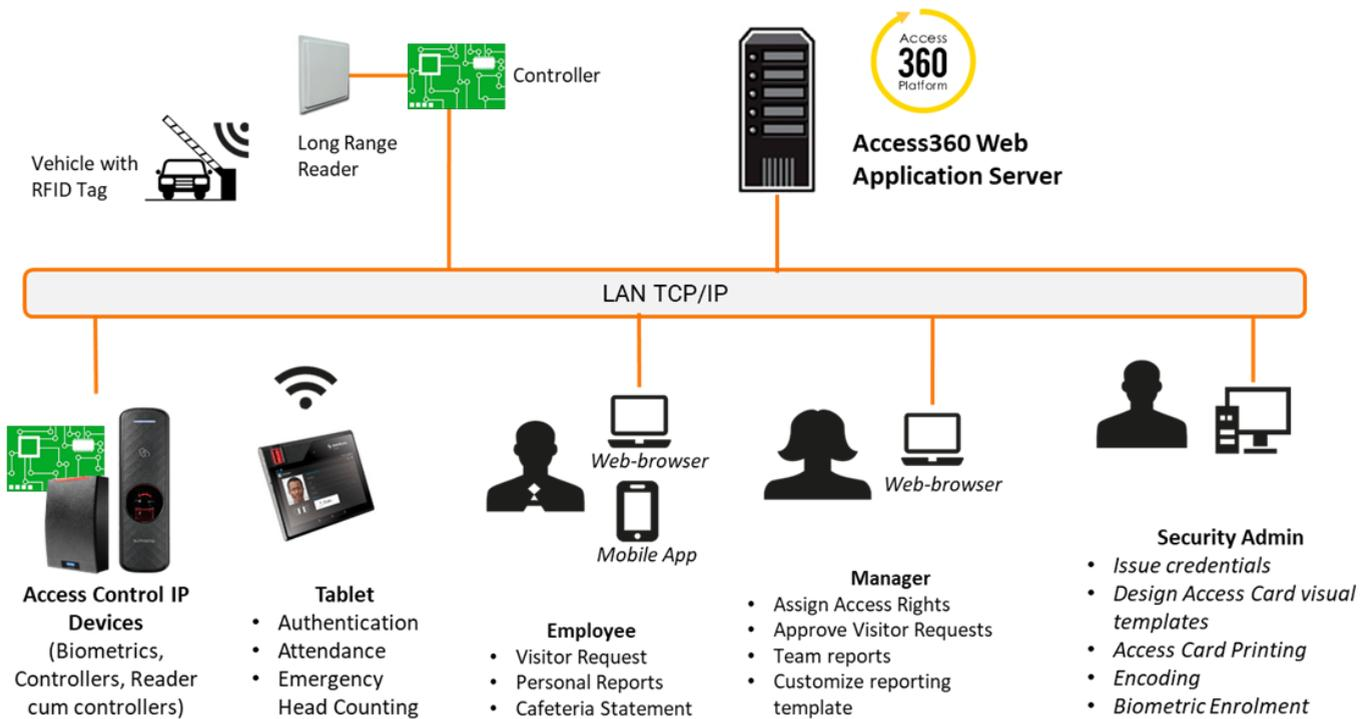
Figure 2: Access360.HRView Access Control System Architecture
